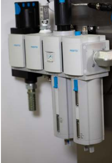
FRL System to Project the Pneumatic System
